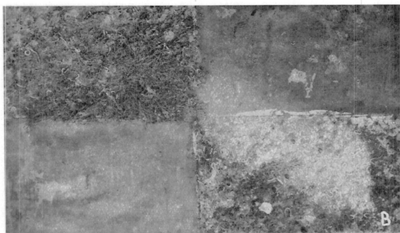
PLATE 6.— A , wood panel, 8.5 × 12 inches, in sea 67 days: Areas coated as follows: upper left, Superwhite enamel plus 10 grams \text{Cu}_2\text{O} , 5 grams \text{As}_2\text{O}_3 and 5 grams \text{ZnO}_2 per 4.74 fluid ounces; upper right, Kress Lettuce Green enamel, normal; lower left, Yacht Green; lower right, Superwhite enamel, normal. B , Masonite panel, 8 × 12 inches in sea 9 months and 18 days: coatings as follows: upper left and lower right, Superwhite enamel, normal; upper right, Yacht Green, lower left, Copper Red.
