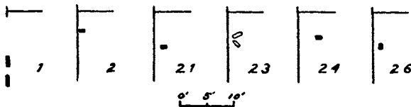
FIGURE 30.—Plans showing position of the uprights on the left rear corner of marae pavements. (Numbers refer to marae, fig. 24.)
