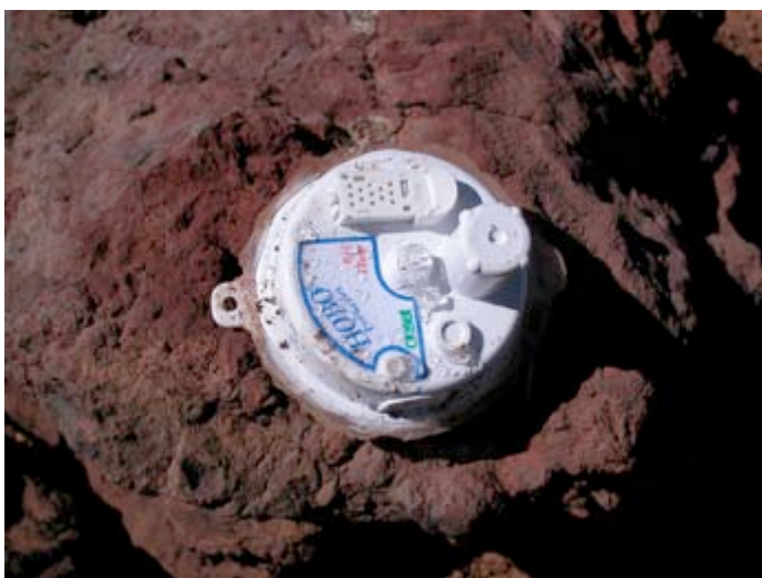
Hobo data loggers used to measure temperature and relative humidities at the Mauna Kea summit.
