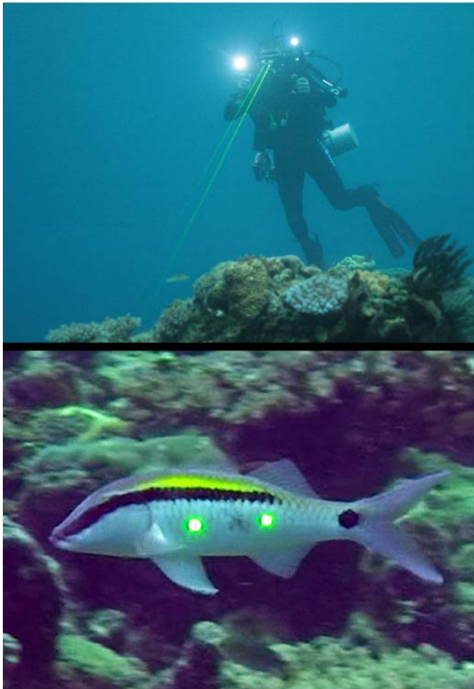
Figure 4. Laser videogrammetry. To estimate fish lengths we have laser pointers mounted in parallel on a video camera used to film fish (top). The lasers superimpose a measuring scale on the side of fish and length can be estimated from frame captures (bottom). Upper photo: Holly Bolick
